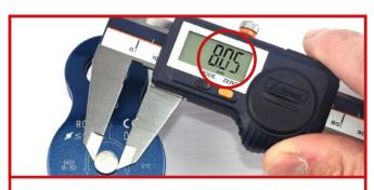
The rivet head has a diameter **smaller than 8.7 mm**: cease to use the pulley immediately and send it to EDELRID for a free replacement.
