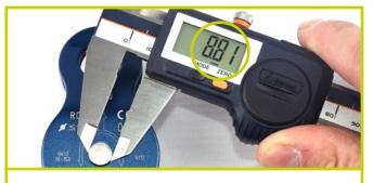
The rivet head has a diameter **larger or equal to 8.7 mm**: the pulley can still be used.
