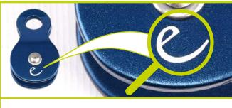
The pulley has a white "e" symbol on the back. The pulley has already been inspected and can still be used.
